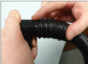
22. Force the outlet hose onto the hosetail. Smear the excess silicone all around the hose connection. We recommend the use of hose clips (not provided).
