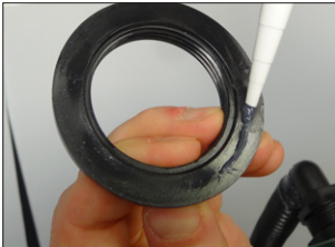
19. Take the nut and place a small bead of silicone around it.
