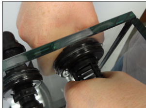
20. Screw the nut onto the bulkhead, now protruding out of the back of the tank. Do it up until it is hand tight. Light pressure from a wrench can also be used to create a tight, water-tight fit.
