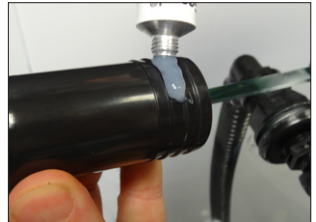
21. Apply a liberal amount of silicone onto the hosetail before offering up the outlet hose.
