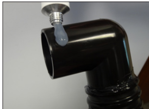
23. Apply a liberal amount of silicone onto the elbow before and insert it into the bulkhead. The elbow and hose should be pointing straight down.
