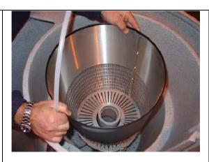
11. Align the air tube as shown, ensuring that the "Eazy" support legs are positioned equally either side of the waste drain.
