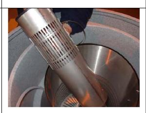
13. Position the supplied Jubilee Clip (band clamp) at the base of the centre pipe and tighten fully.
