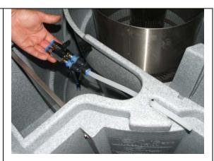
7. Attach the Y Air valve assembly by screwing the self taping screw through the inner chamber into the center of the Y piece
