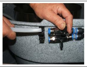
15. Connect the existing air-ring air tube to the lower valve on the "Y" connector.
