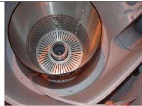
12. Fit the stainless steel centre pipe over the central spigot in the Nexus, aligning the top of the pipe with the top edge of the "Eazy", ensuring that the pipe is vertical.
