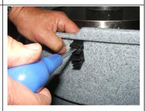
6. Remove the current 90° air-pipe elbow by pushing in the collar and pulling pipe out. Connect the incoming air tube directly to the new "Y" valve system.
