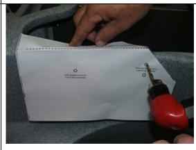
5. Fit the two air-pipe clips using the M4 screws and "Nyloc" nuts supplied.
