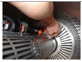
14. Connect the new back wash air tube from the Eazy to the top air valve
