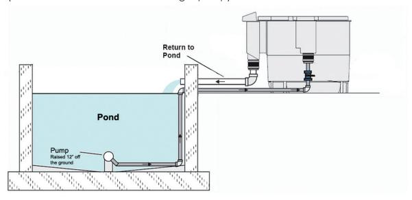
**ARE YOU GRAVITY FED?** By this we mean that your pump is going to be used to return the filtered water to the pond and therefore your filter will be supplied by gravity via a larger diameter pipe. In this situation the water level in the filter will be at the same level as the pond.
