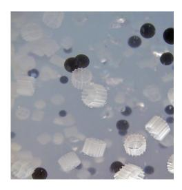
Pure Pond bacteria gel balls in the K1 moving bed filter.
