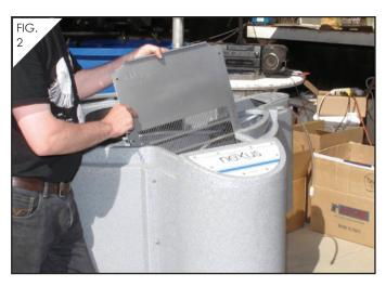
3. Install the new exit screen using the screws provided.
