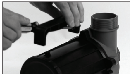
Step 6: Remove the handle.
