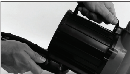
Step 13: Re-fit the base plate.
