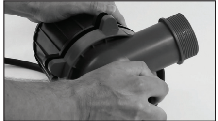
Step 10: Re-fit the impeller housing. This can be positioned at multiple angles.
