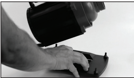
Step 3: Remove the plate from underneath the pump.
