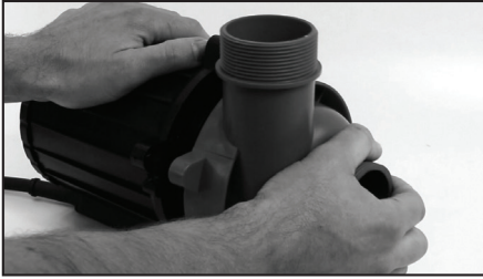
Step 7: Carefully pull away the impeller housing.
