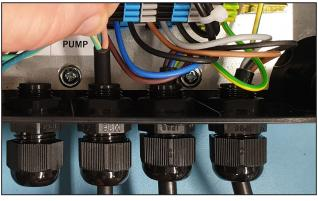
3. PUMP CABLE: Feed enough wire through the gland nut, into the control box to allow you to make the connections to the PUMP terminal block.
