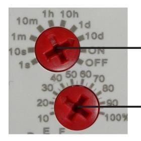
Use a pozi-drive screwdriver to turn the screw head, so the arrow on the dial points to the appropriate digit.
