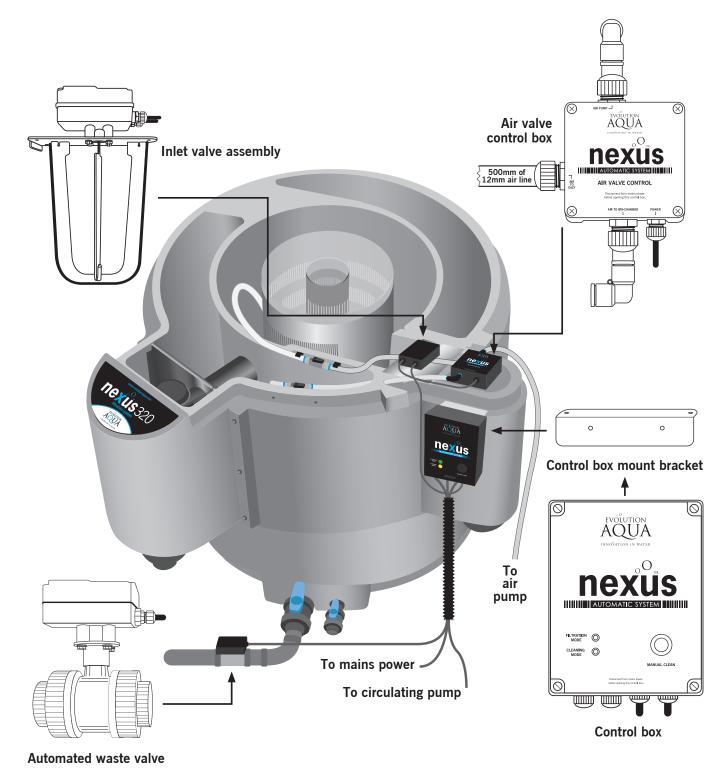
Depending on your installation, it is advisable to fit a non-return valve (not supplied) on your return pipework after the circulating pump. (See page 22)
