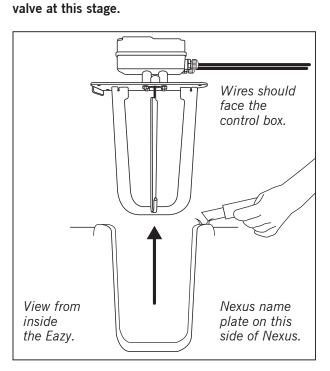
4. Now the 3 holes have been drilled, remove the inlet slide plate assembly. Use a knife or blade to remove any burr or excess plastic from around the holes you have drilled.
