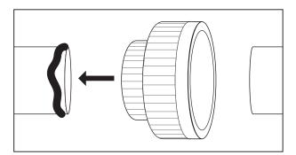
6. Clean and dry the pipe thoroughly. Ensure the union nut is over pipe prior to gluing the insert flange. Apply solvent weld glue to one of the cut ends of the pipe and fit the flange onto the pipe. **TIP: We recommend a "wet and dry" PVC glue be used for gluing the flanges.**
