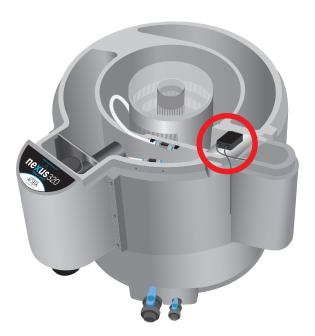
1. The inlet valve assembly should be fitted with the wires from the actuator facing the Nexus name panel and the location of the control box. **NOTE: The inlet valve is supplied in the "OPEN" position. The foam seal should not be fitted at this stage.**
