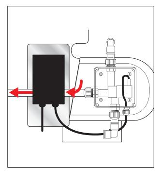
3. Place the Air Valve Control Box as shown. Make sure the air line to the Eazy sits between the Actuator and the stainless steel plate on the inlet valve assembly.
