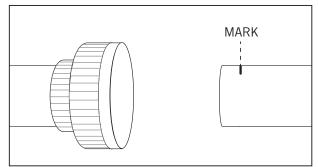
9. Remove the automated waste valve from the pipe.
