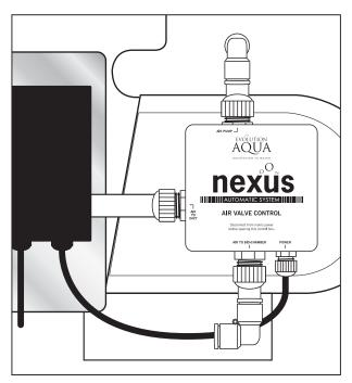
8. The Air Valve Control Box is fitted into position ready for air line installations.
