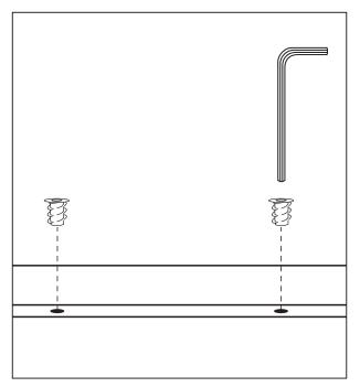
5. Screw 2 fixing inserts into the holes you have just drilled using the 5mm allen key. Tighten inserts until flush with the surface.
