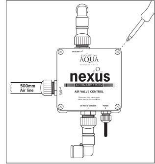
2. Remove the lid off the Air Valve Control Box by unscrewing the 4 screws in each corner of the box to allow access to fixing locations. **NOTE: Keep the 4 screws and O-Rings safe for re-fitting later.**
