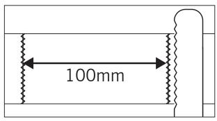
5. From the lines you have marked, cut through the pipework using a saw. Clean and dry the remaining pipe thoroughly.
