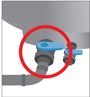
2. Before installation, ensure the waste valve on the Nexus is in a closed position.
