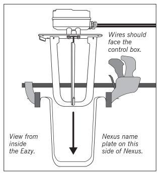
2. In preparation for drilling 3 pilot holes, fit the inlet valve assembly into the correct location. If required, use a sash clamp to squeeze the Nexus inlet together to fit the inlet valve assembly. It may be necessary to drain part of the Nexus to enable easier fitting. **NOTE: The foam seal should not be fitted to the**
