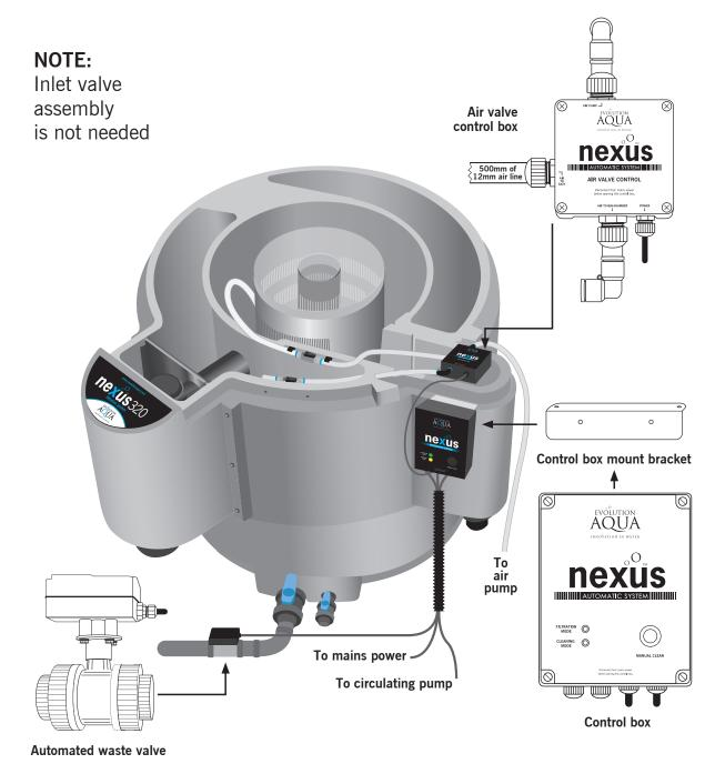
You MUST fit the supplied non-return valve on your inlet pipework after the circulating pump and before the filter. (See page 22 for more details)
