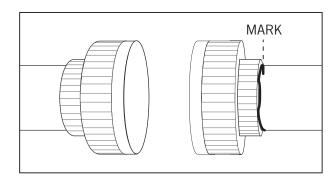
10. Ensure the union nut is over pipe prior to gluing the insert flange. Then, using the mark you made in Step 8 as the guide, glue the flange onto pipe so it is located at this mark.
