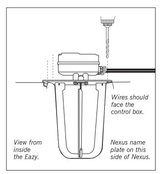
3. With the assembly in position, use the 3 holes in the top of the inlet plate assembly as a guide, and drill 6mm holes through each hole through the body of the Nexus.
