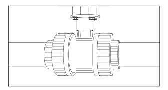
7. Using the automated waste valve as a guide, fit the valve into the glued union end, but do not glue the other union end.
