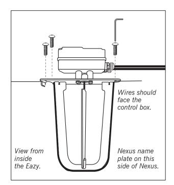
8. Using the 3mm allen key, screw the 3 hex socket screws into the fixing inserts (*PRE-FITTED ON NEXUS AUTO READY MODELS*) and tighten up.
