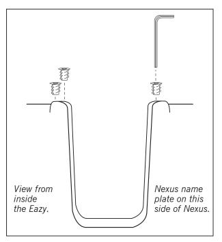
5. Using the 5mm allen key, screw the 3 fixing inserts into the holes you have drilled in the body of the Nexus. Tighten inserts until flush with the surface.
