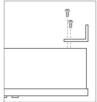
2. Use 2 x 10mm self tapping screws to fit the stainless steel mounting bracket onto the back of the control box to allow the control box to be mounted to the Nexus. (These are the 2 inner holes on the stainless steel bracket that align with the box mounts).
