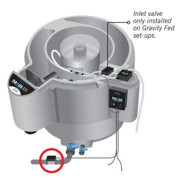
1. You are now going to install the automated waste valve on the waste return pipework from your Nexus. You can position this anywhere that is convenient on the waste pipe run within reach of the power cable.
