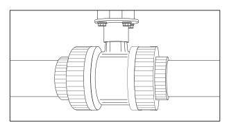
11. Now fit the automated waste valve back in between the union ends and tighten both ends up.
