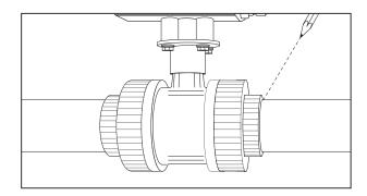
8. Mark the unglued flange position on the pipe with a pencil or marker pen.
