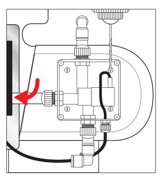
4. To fit the Air Valve Control Box in this position, drill 4 pilot holes using the 3mm drill bit through the 4 plastic panels in the base of the box.
