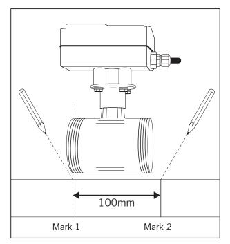
4. Use a pencil or pen to mark the waste pipework in line with one end of the ball valve minus the end cap. Then measure 100mm along the pipe and make a second mark.
