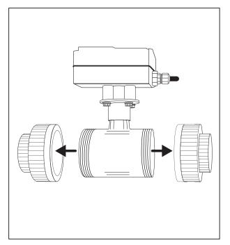
3. Taking the Automated Waste Valve, unscrew both union ends off the automated waste valve.
