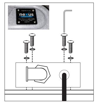
6. *IF YOUR NEXUS IS AN AUTO READY MODEL*, use the allen key provided to remove the screws from the acrylic information panel on the inlet. Discard the acrylic panel. Then use the same hex headed screws to install the the air valve control box.
