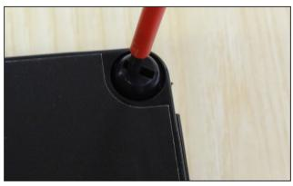
1. To open the box, use a flat head screwdriver to unscrew the plastic screws on the box. The lid can open to 90° with 2 loose screws. **DO NOT FORCE THIS OPEN.**
