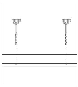
4. Move the control box away and then drill 2 holes into the positions you have marked using a 6mm drill. You may need to use a knife to remove any excess plastic or burr from around the holes you have drilled.
