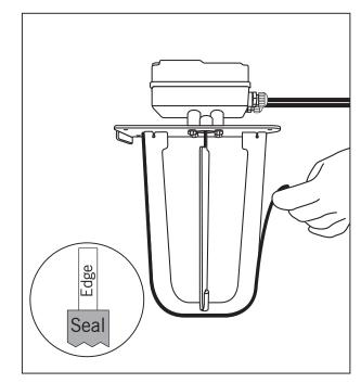
6. Ensure all edges of the inlet valve assembly are completely dry. Peel off the backing tape from the foam seal, then proceed to fit the foam seal around edge of the outer blade on inlet valve assembly. The seal must be centrally aligned. Trim off any excess length.
