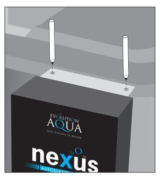
3. Hold the Nexus Automatic control box in the position you want it located on the Nexus. Now use a marker pen to make 2 marks where the screw holes are on the stainless steel bracket.
