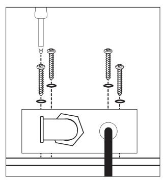
5. When all 4 pilot holes have been drilled use the 25mm screws and O-Rings provided, to screw the box onto the Nexus. Use a pozi drive screwdriver to tighten the 4 screws up.
