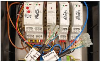
2. With the box front open, familiarise yourself with the connectors inside. The pump and mains cables are fitted with terminal blocks for easier connection to your pump and mains supply.
