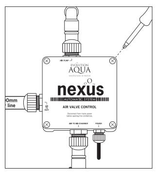
7. Use the 4 screws and O-Rings you removed in Step 2 to tighten up the lid on the Air Valve Control box.
