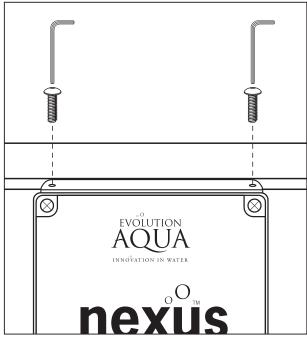
6. Fix the control box onto the Nexus using the pan head hex socket screws and the 3mm allen key. (PRE-FITTED INSERTS ON NEXUS AUTO READY MODELS)
