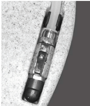
Air Valve On
