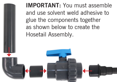
Figure 7.1. Hosetail assembly
