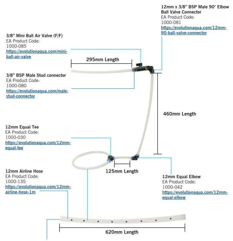
Holes for the air ring need to be 60mm apart and there should be 9 holes in total as shown above with holes being 4mm in diameter.
