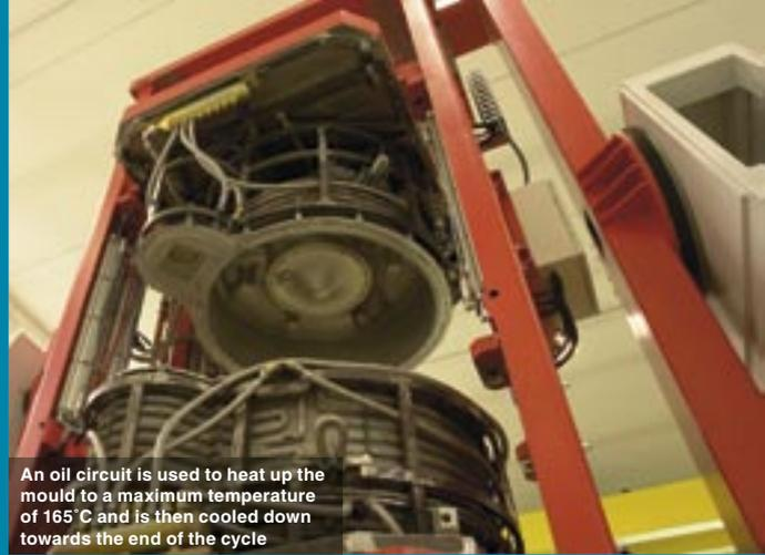
An oil circuit is used to heat up the mould to a maximum temperature of 165°C and is then cooled down towards the end of the cycle
