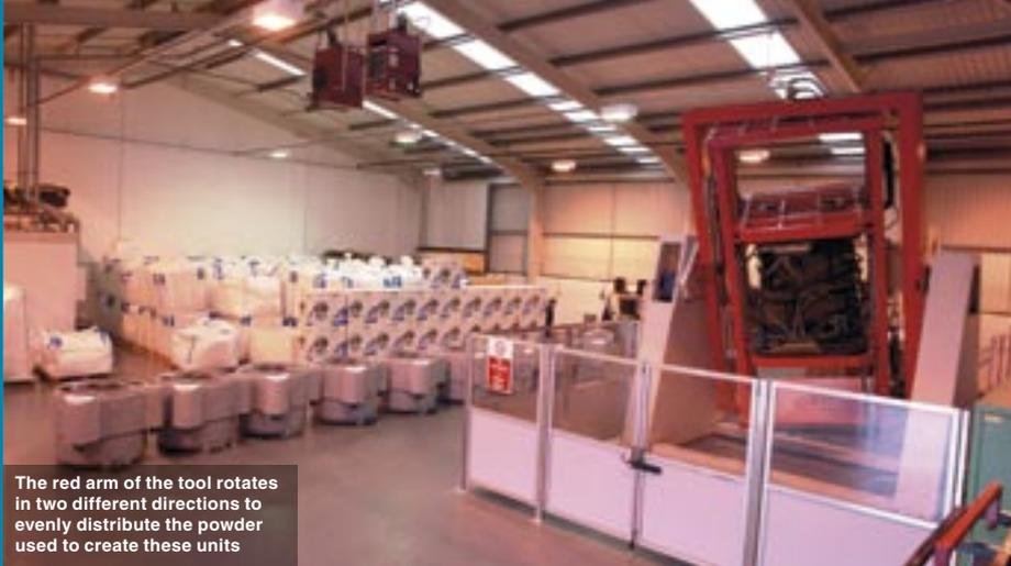
The red arm of the tool rotates in two different directions to evenly distribute the powder used to create these units
