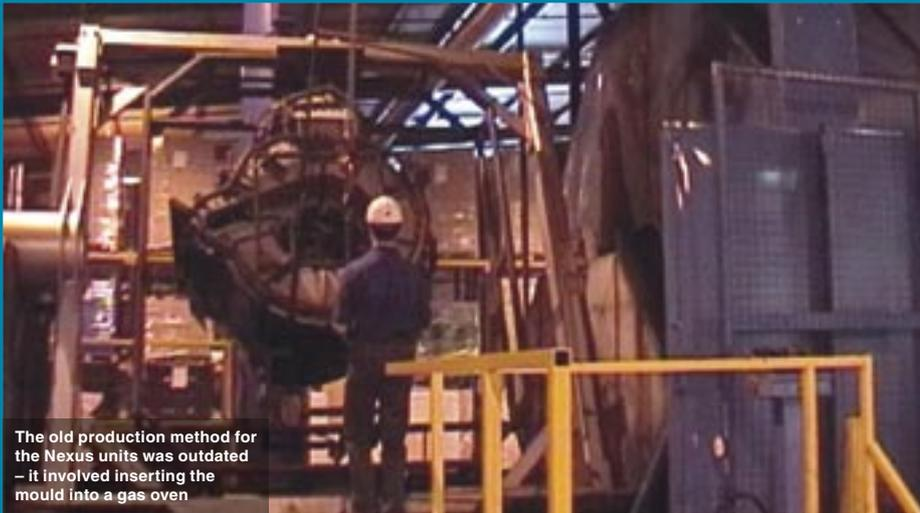
The old production method for the Nexus units was outdated – it involved inserting the mould into a gas oven
