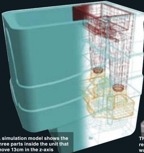
A simulation model shows the three parts inside the unit that move 13cm in the z-axis
